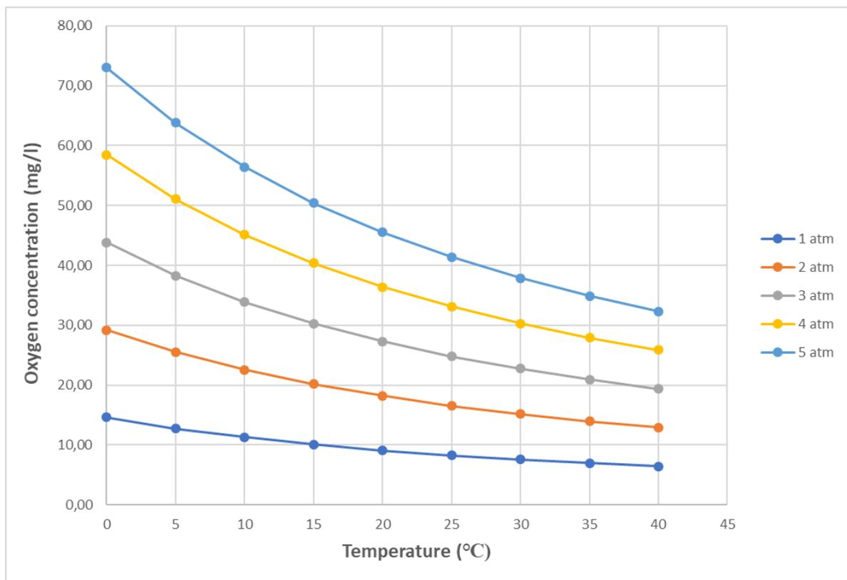
Figure 1 Physical oxygen holding capacity of fresh water as a function of temperature, demonstrated for several water pressures. Salinity of the water is not taken into account here, but typically negatively influences the physical oxygen holding capacity of the water, e.g. for water at 1 atm with EC of 1.7 the holding capacity lays on average 2-3 ppm lower.
